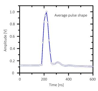
Average pulse shape was acquired as an average of 100 000 analog pulses (directly from amplifier) with amplitudes 1 V  $\pm$  0.05 V. For this purposes, the NI USB-5133 digitizer was used.
